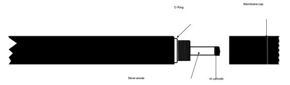
The electrolyte will have absorbed oxygen during storage (more so if the bottle is becoming depleted). This dissolved oxygen in the electrolyte will have to be scavenged out before readings will have any accuracy.
