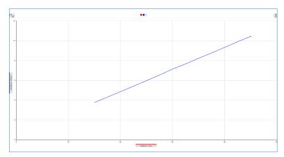
It would be surprising with a metre length to get an exact match to specification. Resistance at junctions between the jockey and wire and crocodile clips will create an off set in the data.
