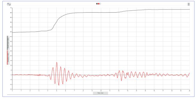
Use the difference tool to find the time interval between the start of the initial noise and the start of the echo. You may need to discuss with others about exactly were you will measure from to. If you look carefully at the dBa data you will see a slight uptick in the data that lines up with the echo, you can use this to get a more precise start point to the echo.
