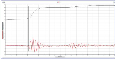
Difference tool use to identify the start of the two sound pulses. With the echo the slight uptick in the dBa curve has been used to find the start of the echo.
