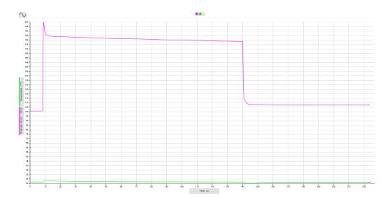
You will need to find and record the pressure and volume of the syringe at the same temperature with and without compression of the gas. The volume will be the initial volume of the syringe and the volume when the plunger is pushed to the stop. The pressure is the pressure before compression and when the temperature falls back to the start temperature with the gas still compressed.
