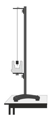
The pendulum was the controlling mechanism for the first accurate clocks. Until the pendulum properties were discovered we did not have clocks that could measure time with any precision. The pendulum period (time taken to move through one "swing") is independent of its swing amplitude (the distance of the swing). How does its period vary as you change the length of the pendulum?
