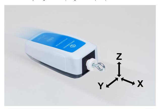
The gyro produces a +ve reading for clockwise rotation and a -ve reading for anticlockwise rotation.
