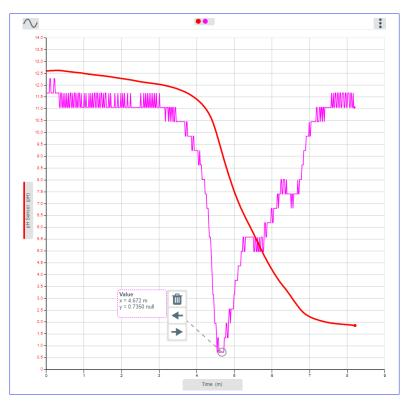
First derivative graph, the mathematical application amplifies positions where data does not change and shows many erratics. But it is obvious where the peak of greatest change of pH is taking place and the local point tool can be used to find the volume.
