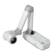
The mechanical body structure allows the camera to rotate 90 degrees vertically and horizontally so it can also be used as a webcam to capture classroom activities or for videoconferencing. Capture, store and present images with an SD card or computer.
