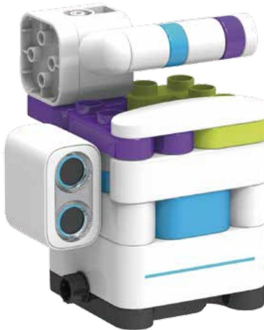
Let's build a smart trash bin, the cover of the trash bin can open and close when the sensor is triggered.
