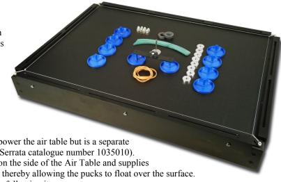
An adjustable speed air blower is available to power the air table but is a separate item not supplied as part of the air table (refer Serrata catalogue number 1035010). The blower is connected to the air inlet found on the side of the Air Table and supplies air to the many small holes in the table surface thereby allowing the pucks to float over the surface. An accessory set is supplied which contains the following items:
